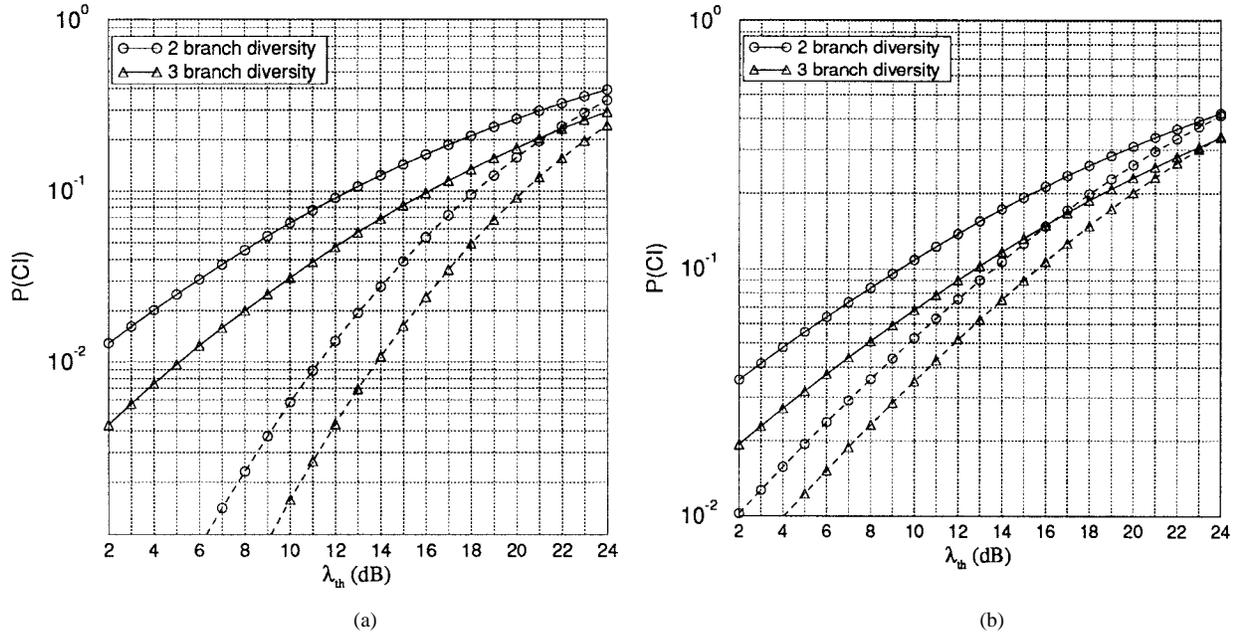
Fig. 2. The CCI probability  $P(CI)$  against the required threshold  $\lambda_{th}$  at the receiver for the local-mean-based macrodiversity system over (a) pure shadowing channels and (b) shadowed Rayleigh channels, where the solid lines (—) denote the case for shadowing standard deviation  $\sigma = 10$  dB and the dashed lines (- - -) for  $\sigma = 6$  dB and  $a = b = 2$  and  $g = 0.15R$ ; two interferers are located at a distance of  $5.2R$ .
