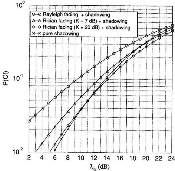
Fig. 1. Comparison of CCI probability  $P(CI)$  for no macrodiversity over pure shadowing channels, shadowed Rayleigh channels, and shadowed Rician channels, where  $\sigma = 6$  dB and  $a = b = 2$  and  $g = 0.15R$ ; two interferers are located at a distance of  $5.2R$ .
