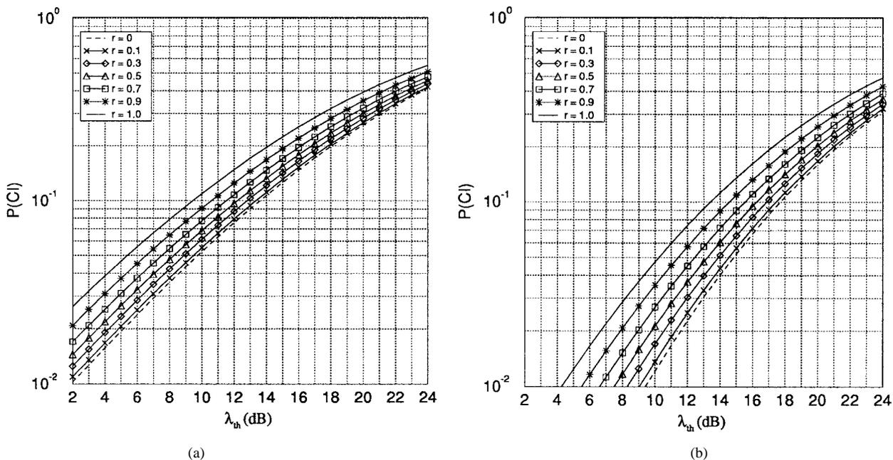
Fig. 4. Effect of branch correlation coefficient  $r$  on the local-mean-based macrodiversity system with Rice factor (a)  $K = -\infty$  dB and (b)  $K = 10$  dB, where  $\sigma = 6$  dB and  $a = b = 2$  and  $g = 0.15R$ ; two interferers are located at a distance of  $5.2R$ .
