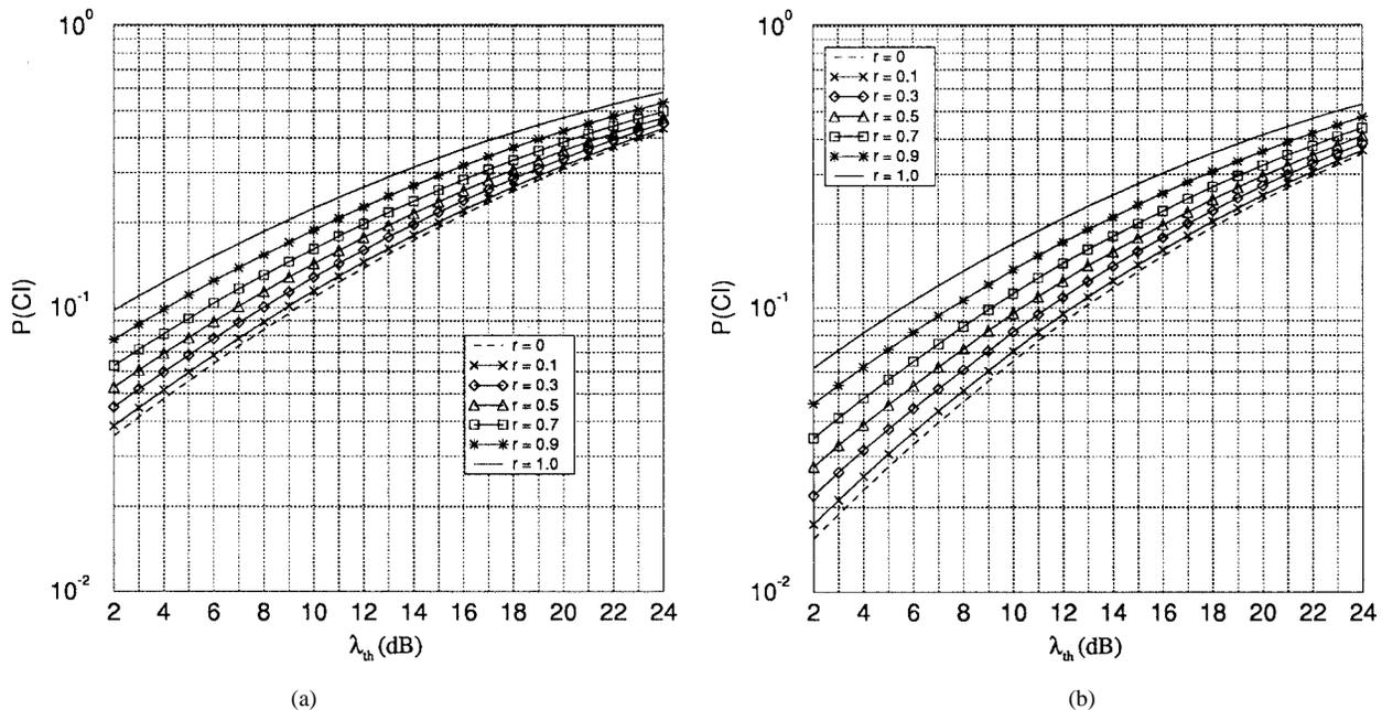
Fig. 5. Effect of branch correlation coefficient  $r$  on the local-mean-based macrodiversity system with Rice factor (a)  $K = -\infty$  dB and (b)  $K = 10$  dB, where  $\sigma = 10$  dB and  $a = b = 2$  and  $g = 0.15R$ ; two interferers are located at a distance of  $5.2R$ .
